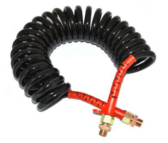
• The connector is used to connect the pneumatic brake system of the vehicle with the trailer system
